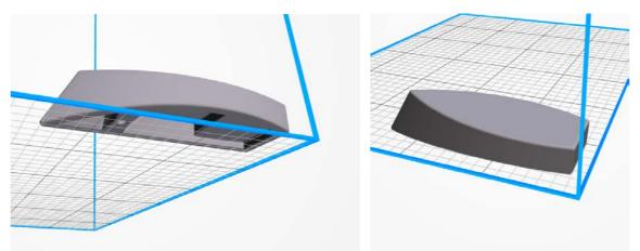
If we print the part with the orientation shown above, we will see the difference between layers in the surfaces that have an angle less than 20<sup>o</sup> to the horizontal plane:
