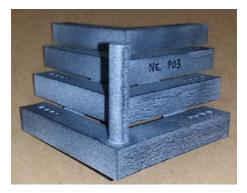
Elephant skin is due to not properly controlling the bed temperature; this can be avoided by cleaning the Fusing and Heating lamp glasses and the Temperature camera glass.
