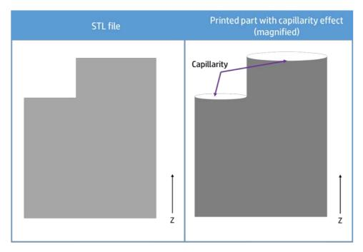
Orient the part correctly in order to minimize its top surface area, to reduce the visibility of the defect.
