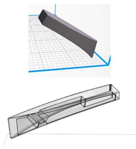
As can be observed in the figure above, the hole to insert the sail won't be printed along the XY plane, where the best resolution is achieved. This is a trade-off that we must accept in order to maximize the part's look and feel.
