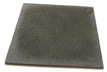
Orienting the part correctly in order to minimize its top surface area is the key to completely neutralizing the possibility of this defect. This picture below shows the same part after being printed with an inclination of 45° to minimize its top surface area.
