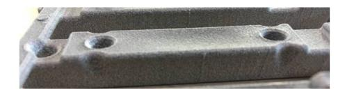
For parts that are thick and dense you might experience a local shrinkage on the surface of the part. This is more frequent on top surfaces.
