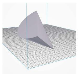
In the figure above you can see that the part is also placed in order to prevent stair-stepping (avoiding angles less than 20 degrees to the horizontal plane) by placing the curves upside down.
